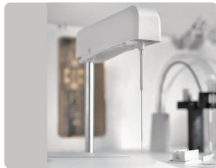
Intelligent probe with optional clog detection
