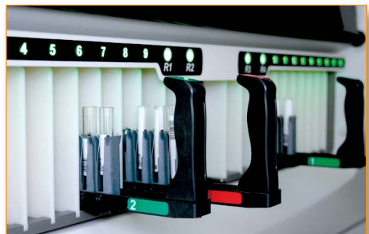
Sample loading area for up to 180 samples and 28 reagents
