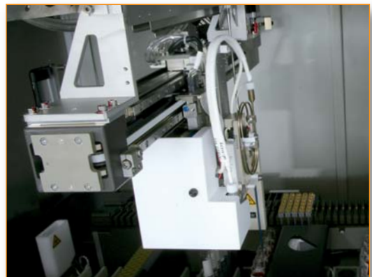
2 independent pipetting arms, separate transport arm for cards
