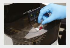
In the carousel mode, single sample tube can also be loaded as STAT after opening the cap of carrousel.
