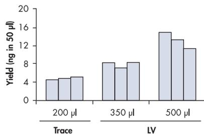
**Figure 6. Higher yields of concentrated DNA with the large-volume protocol.** DNA was diluted in Buffer G2 to a final concentration of 50 pg/µl, and the indicated volumes were processed using the EZ1 DNA Investigator Kit with the standard trace protocol (**Trace**) or the large-volume protocol (**LV**). All samples were eluted in 50 µl water, and 5 µl was quantified using real-time, quantitative PCR.
