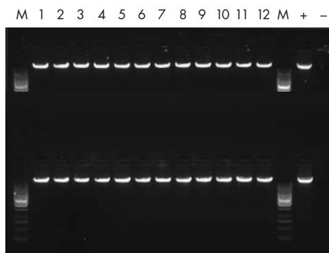
**Figure 1. Reproducible high-quality DNA.** Genomic DNA purified from whole blood. Upper lanes are from 200 µl blood, lower lanes are from 350 µl blood. Lanes 1–6 and 7–12 are from the first and last of 8 processing runs on the EZ1 Advanced workstation, respectively. **M:** 1000 bp DNA ladder (100 ng); **+**: positive control; **-**: negative control. A 2 µl aliquot (1%) of each eluate was visualized on the agarose gel.
